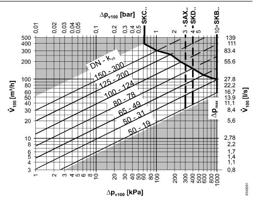
$\Delta p_{\text{max}}$  = Maximum permissible differential pressure across the valve, valid for the entire actuating range of the motorized valve
