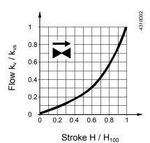
$\begin{array}{ccc} 0...30 \; \% & \rightarrow & linear \\ 30...100 \; \% & \rightarrow & equal \; percentage \\ & & n_{ql} = 3 \; as \; per \; VDI \; / \; VDE \; 2173 \end{array}$
