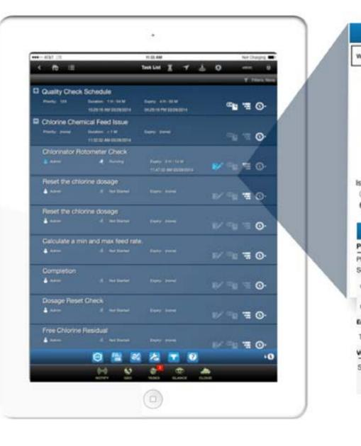
Fourth-generation HMI/SCADA also bridges the gap between operations and maintenance. When an out-of-spec event takes place in the SCADA, operators can trigger a work process to interface with the CMMS/EAM system, secure a work order number, send specific instructions including GIS location, and facilitate corrective action to remediate the problem.
